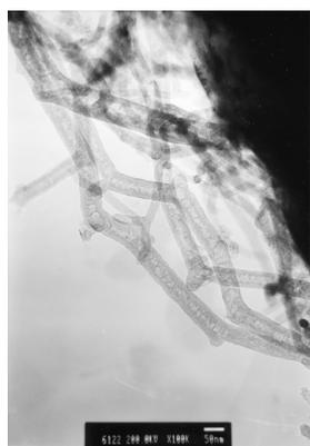
Figure 3. Y-junction structure of CNT obtained in area (3).
