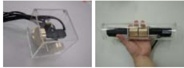
Fig 3. (Left) Developed 3D-GyroCube, and (Right) TwinMotors GyroCube.
